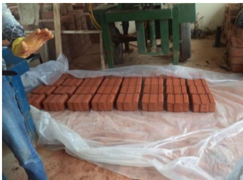
Plate 1: Stacking and Curing of Blocks
