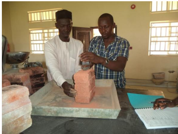
Plate 5: Determination of the Abrasive Strength of NBBRI CSEB
