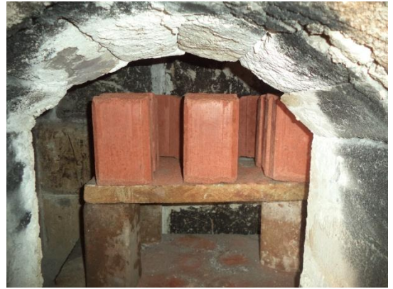
Plate 2: NBRRI CSEBs Samples arranged in Kiln for Firing
