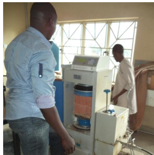
Plate 4: Testing the Compressive Strength of Block sample
